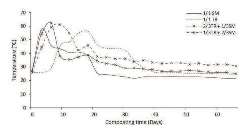
After the addition of each mixture in the bioreactor, increasing in temperature was observed in all treatment, indicating a marked microbial activity. In composters containing the controls CTPR (Tomato plant residues) and CSM (Sheep manure), the thermophilic phase (up to 47°C) lasted 15 and 5 days respectively for CTPR and CSM. The maximum temperature inside of
